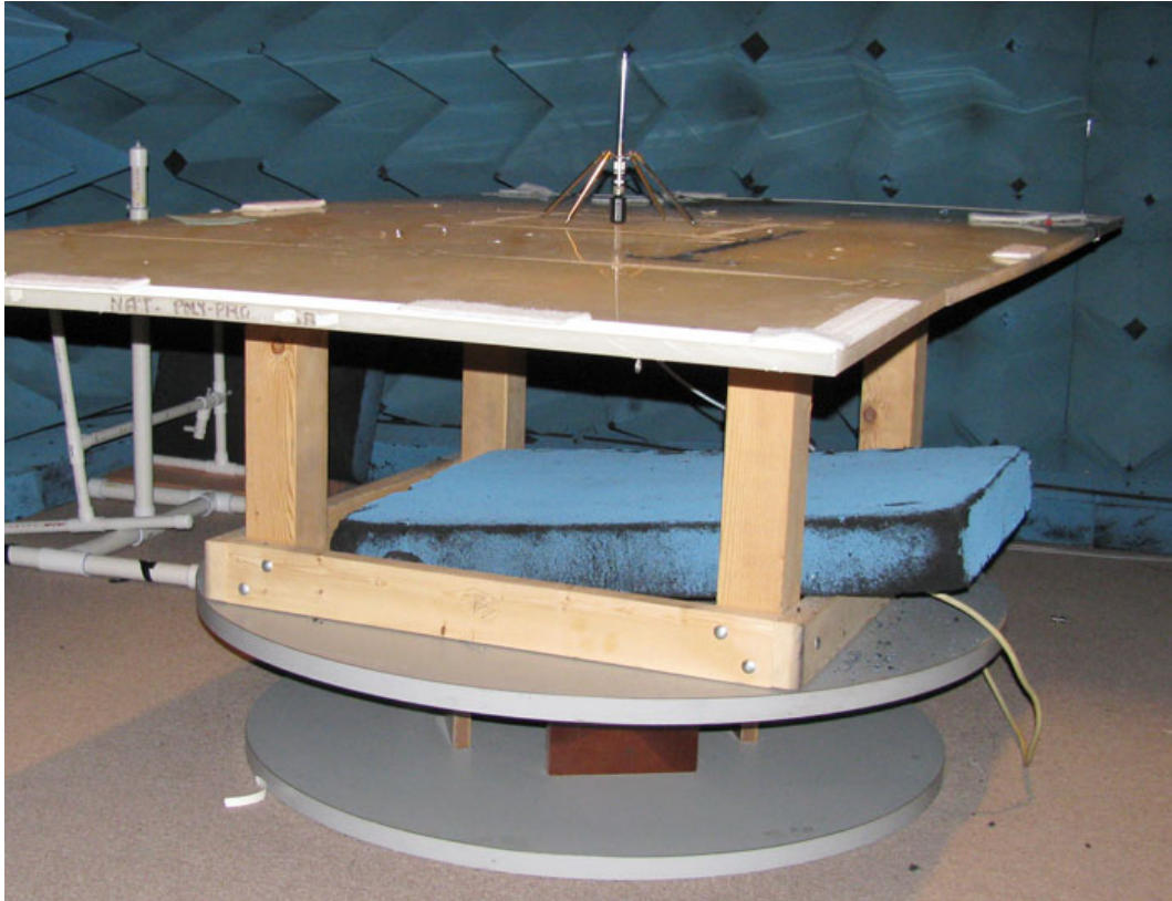
Fig. 4 - Comb generator and antenna installed into a 3m chamber. The comb generator and it's USB power supply were buried under the carbon-loaded foam block. Several ferrite chokes were installed at intervals along the power and coax cables. One of these chokes can be seen at the base of the antenna.
