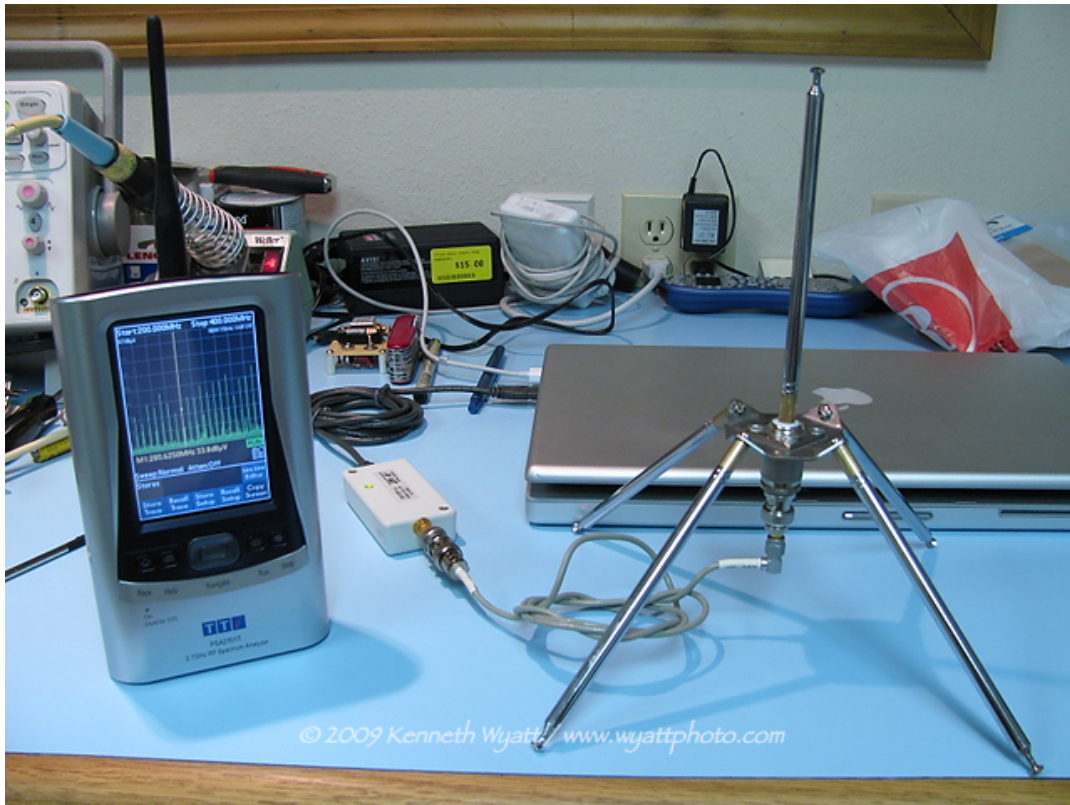
Fig. 3 - Reference antenna used for comb generator testing in the 3m chamber. I'm not sure of the source for this antenna, as it was given to me as a retirement gift by another ham/employee. The elements are telescoping, but I used it in the collapsed state.
