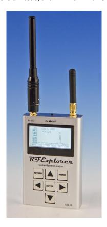
Here's the "RF Explorer - WSUB3G", a handheld spectrum analyzer that sells for \$269 and covers 15 MHz to 2.7 GHz.
