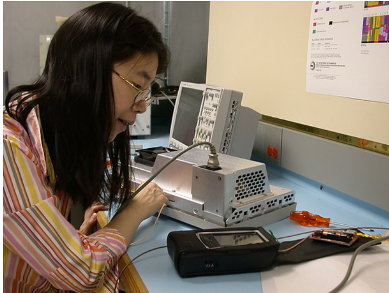
Figure 3 - Here, engineer Yuan Ma, scans a product for mechanical leakage between adjacent pieces of sheet metal. She's using the PSA1301T (1.3 GHz) analyzer with the Mini-Circuits wide-band preamp and Beehive H-field probe.
